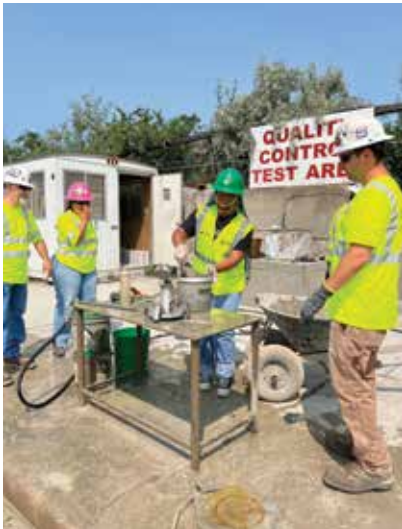
A Polished Pebbles participant performs an air content test using the pressure method. The group learned about a variety of tests.
