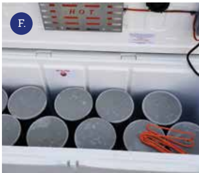
Figure 1: Casting and curing of cylinders
