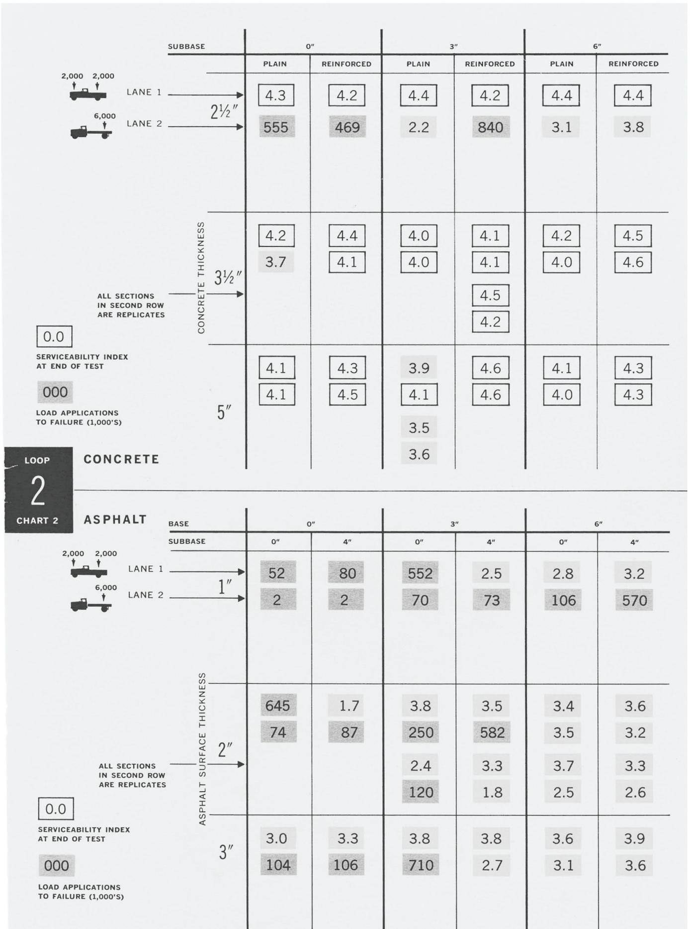
The tables in *Figure 1* demonstrate how the pavement sections performed. The tables are a little busy, but they are jam-packed with exciting information for pavement geeks interested in promoting concrete pavements for parking lot applications.
