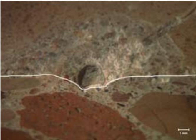
**Fig. 1:** Popout due to alkali-silica reaction (photographed at an angle). The white line delineates the boundary between the top surface (above line) and the polished surface perpendicular to it (below line). The offending shale particle can be observed in the base of the popout.
