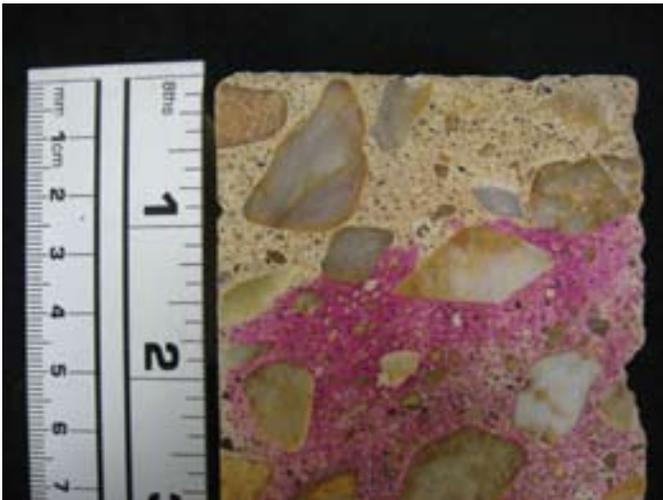
**Fig. 3:** Phenolphthalein turns deep pink [darkly shaded area] if the pH is above about 9.5. The upper photograph shows a concrete with negligible carbonation, whereas the lower photograph shows a concrete that is heavily carbonated.
